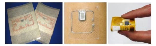
While most of epidermal electronics is intended to be coupled with low-frequency coils for communication with a mobile phone in the very near field (few centimeters read-distance, at most), integrating epidermal sensors with higher-frequency antennas will instead extend the wireless interaction with the skin up to some meters. Biophysical parameters can be automatically collected by the surrounding environment thus enabling the seamless connectivity of human bodies to the Internet of Things.
