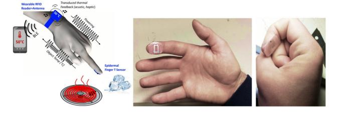
Radiofrequency Finger Augmented Devices (R-FAD) combine the advanced flexible electronics typical of FADs tools with wireless communication based on passive backscattering (UHF RFID) to turn the human fingers into enhanced sensory interfaces aimed at restoring lost peripheral sensitivity in people affected by *Hypoesthesia*, and even expanding their senses beyond natural ones (*ultrability*).
